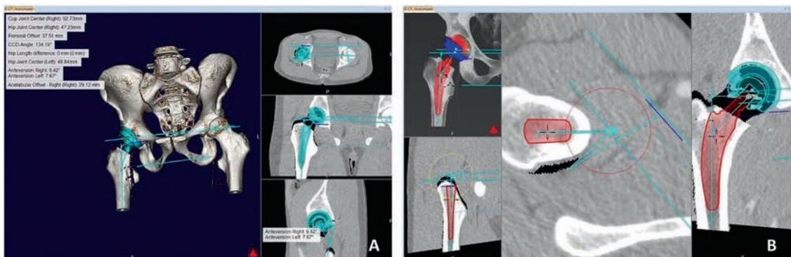
**Figure 1 – 3D-CT planning with a dedicated software package (mediCAD©, HecTec GmbH). A) Most if not all THA planning software have 3D reconstruction functionality and allows positioning of the acetabular component on the axial, coronal and sagittal 2D views. B) This is also possible with stem anteversion and position of the femoral head.**
